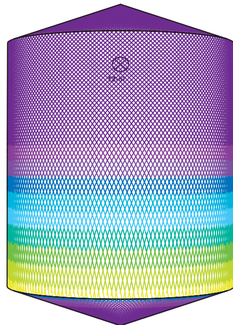
D2.5m H6m, Toftejorg TZ-67, 4 x 6 mm Time = 14.7 min., Water consumption = 3097 l
