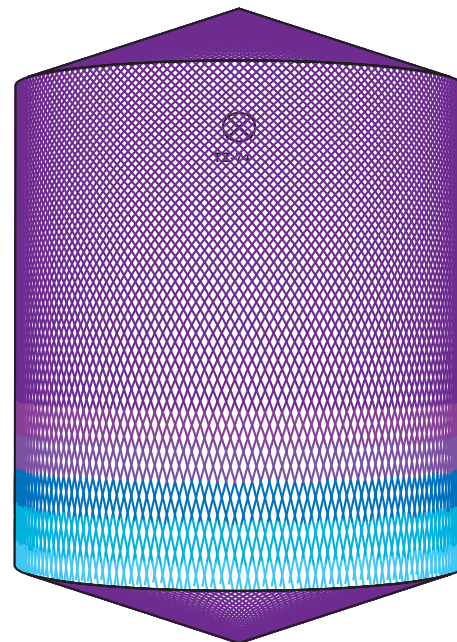
D5m H6m, Toftejorg TZ-74, 4 x 7 mm, 0% Time = 19 min., Water consumption = 5408 l
