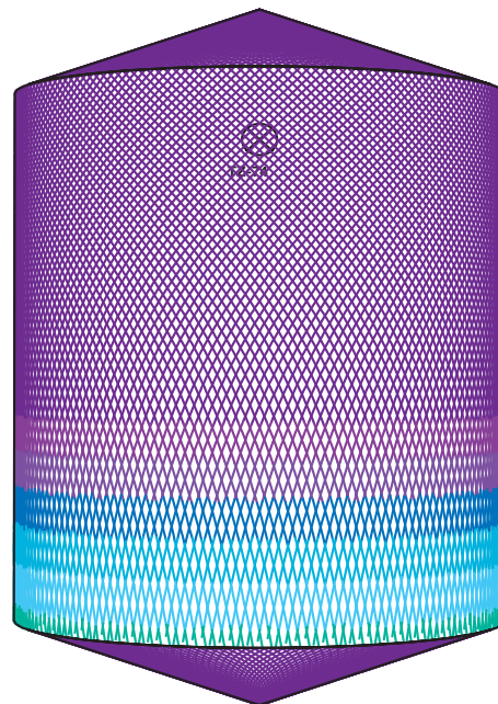
D5m H6m, Toftejorg TZ-74 Self Cleaning version, 4 x 7 mm, 0% Time = 15.3 min., Water consumption = 4853 l
